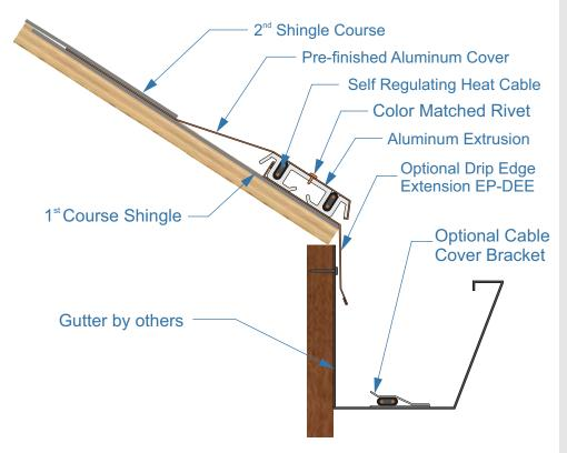
**NOTE:** Some roof assembly features omitted for clarity. IceBlaster products are fully compatible with most roof styles and systems. IceBlaster <sup>™</sup> Eave Panel can be installed on a roof overhang without a gutter. Cable Cover Bracket (CCB) is optional. Optional Drip Edge Extender can be used when no drip edge is present or when the EP-SO must be positioned further up on the roof. The Drip Edge Extender provides for heat transfer on the roof edge.
